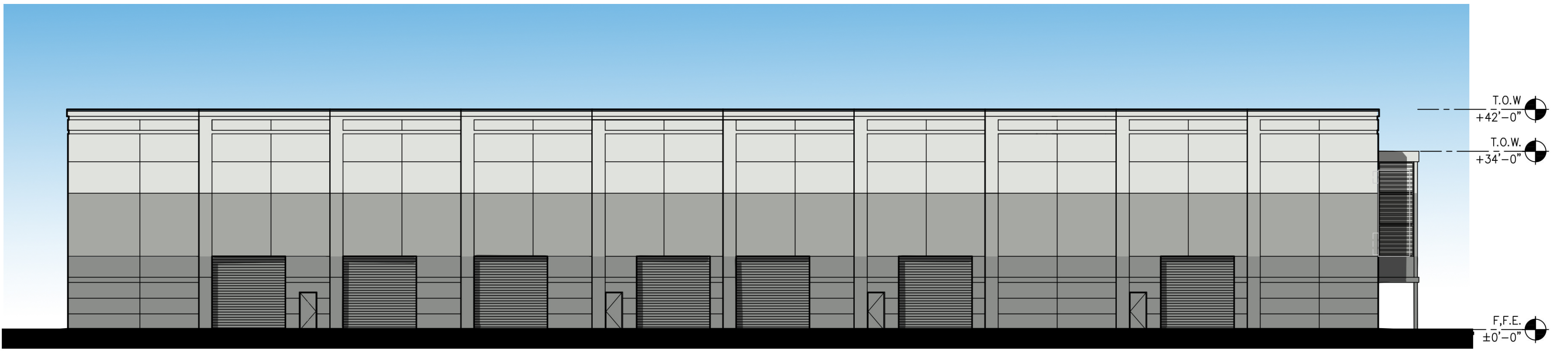
EAST EXTERIOR ELEVATION - BUILDING 2 SCALE: 1/16" = 1'-0" 3
